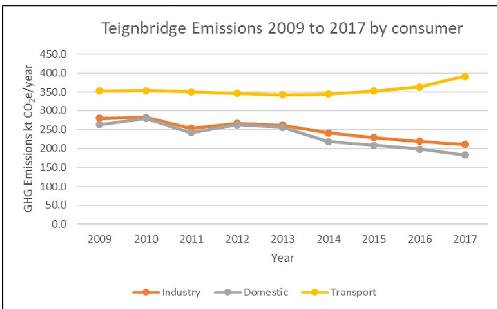
The main reason for the drop in emissions from the domestic and industrial sectors shown above is the reduction in emissions from electricity generation. There is limited scope for a further reduction, except by substituting electric vehicles (EVs) for those powered by fossil fuels.
